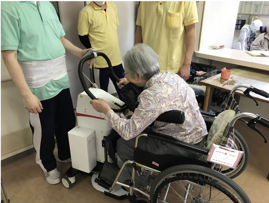
Figure 1. The Hug in action. The carer on the left who is operating the Hug is wearing a support belt after suffering a herniated disc, which he attributed to transferring residents. Photograph by James Wright.
